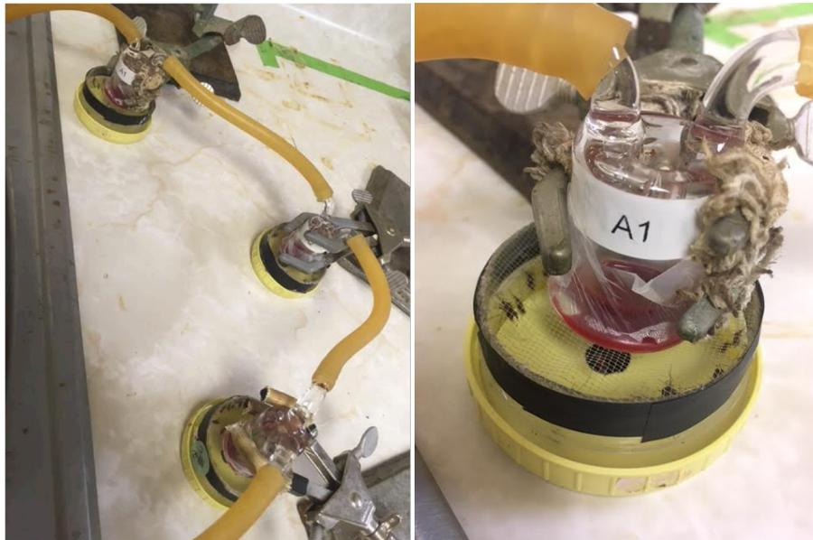
Fig. 2. Rutledge feeders and tubing held by utility clamps.
