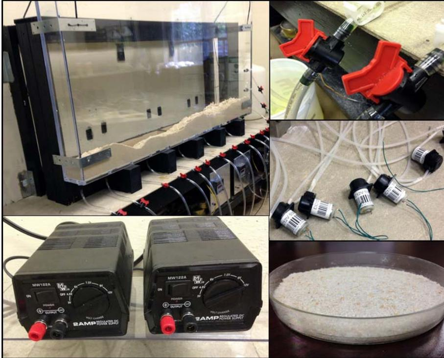
Figure 17. The physical model, power supplies, valves, pumps, and sand counter clockwise from left to right.
