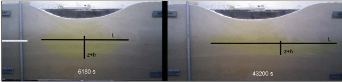
Figure 29. Simulation showing lens degradation and lateral flow in the direction of the gradient.
