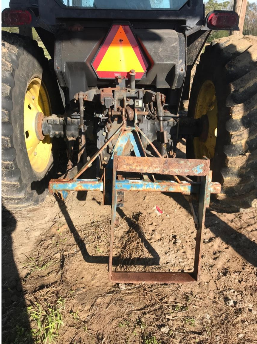
Figure A.1. A steel frame constructed to fit a three-point tractor hitch to cut alfalfa roots at approximately one meter for carbohydrate analysis at the University of Georgia Animal and Dairy Science farm in Tifton, Georgia.
