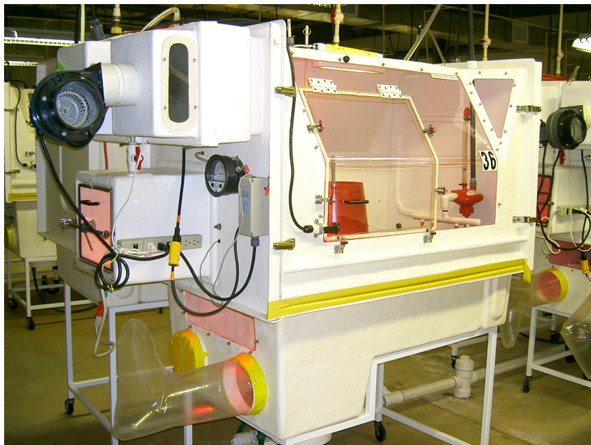
Figure 4. Isolator units (Controlled Isolation Systems Inc., San Diego, California) used in the experiment (image by Thitaram, S.N.)
