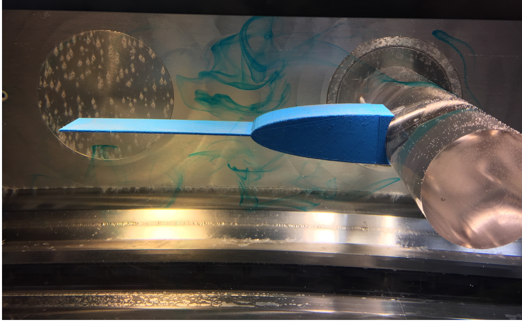
Figure 3.1. A cantilever beam with a chord length of 15.24 cm, span of 5.08 cm, and thickness 2.54 mm stationed behind a horizontally mounted cylinder with a diameter of 7.62 cm located in the test section of a water tunnel.
