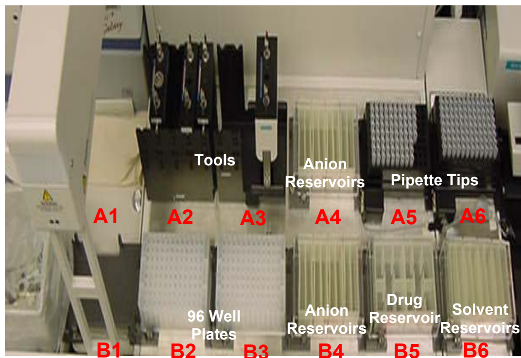
Figure 4.6. Automated Trazodone Salt Formation Setup of Labware on the Worksurface of the Biomek 2000 Workstation
