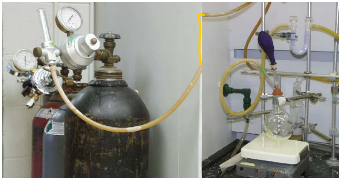
Figure 2.9. Dry Nitrogen Purge and Evacuation Setup for Orthoester HPMA Reaction
