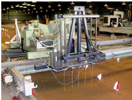
Figure B 2.6 Soil cone penetration reading using multiple-probe soil cone penetrometer on the Norfolk sandy loam soil bin at the USDA-ARS- NSDL facility in Auburn, AL.
