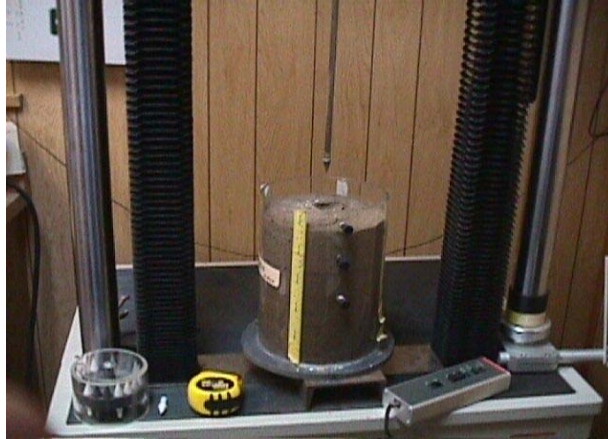
Figure A 2.3 Soil cone penetration reading using Sintech/2G at the USDA-ARS- NSDL facility in Auburn, AL precision farming lab.
