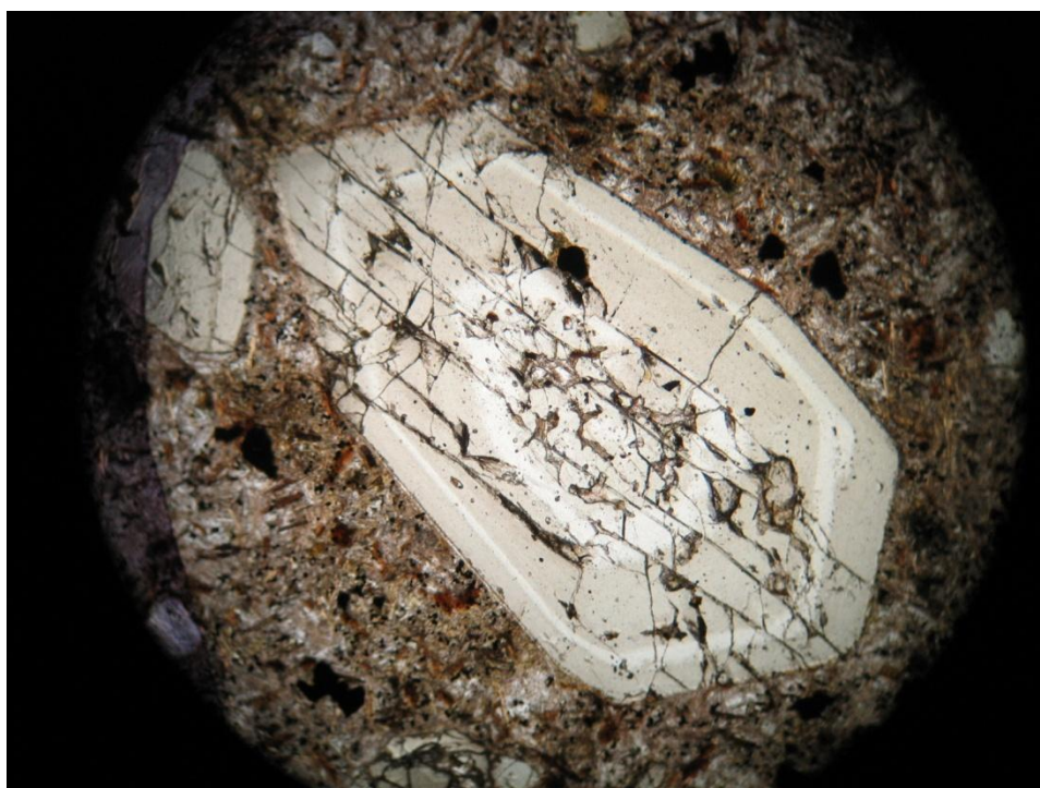
Figure 3.2) Light photomicrographs of 11-AMS-06 Cpx 9. Cross polarized and plane polarized light, field of view is ~5 mm in diameter.
