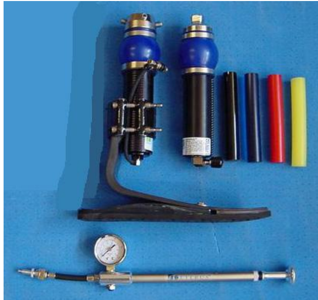
Figure 1.1 Ceterus © SAP attached to the Re-Flex © foot (top left); Ceterus components (top right), and the air pump (bottom). One of four viscoelastic rods (top right) are placed into the black tube of the SAP (left of rods). The pump is used to adjust the air pressure in the blue bulb of the SAP.
