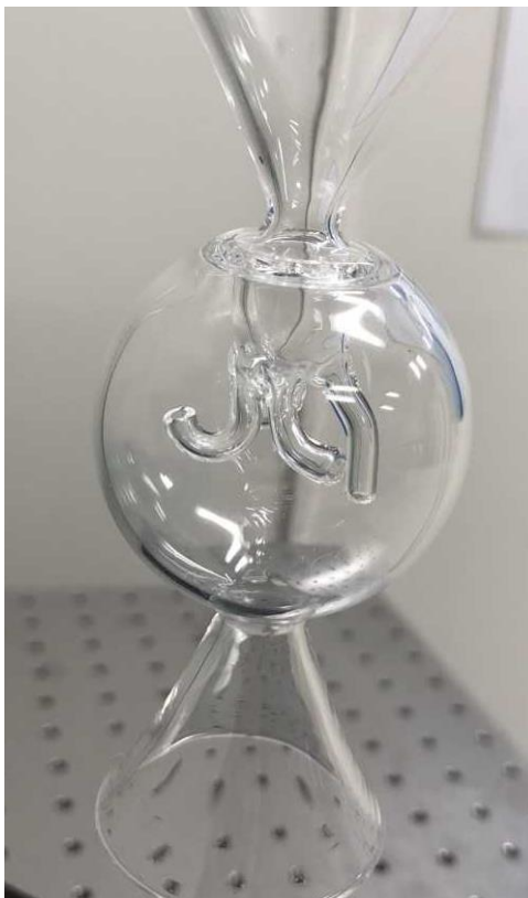
Figure 3: Four turbulent jets are used to provide secondary mixing inside the spherical reaction volume.
