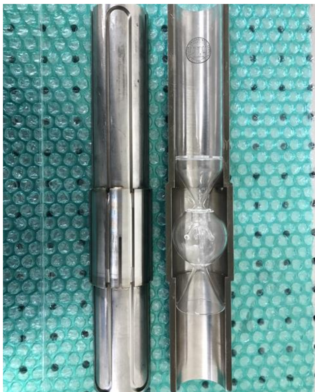
Figure 28: Ridged Inconel body with grooves for heating elements
