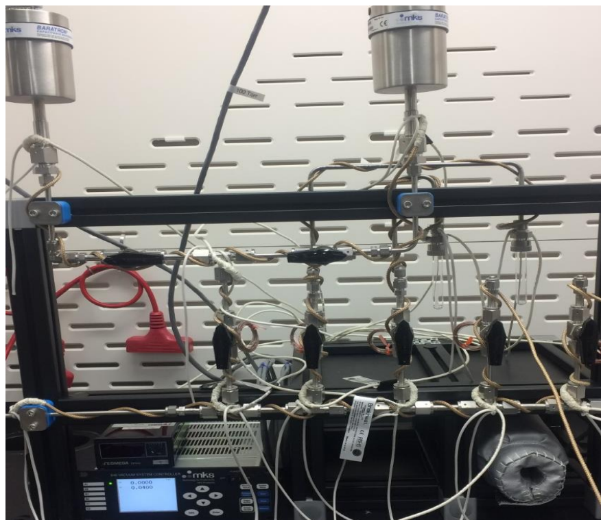
Figure 18: Manifold used to create gas phase mixtures of hypothesized products at known concentrations
