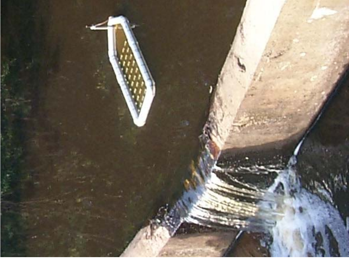
Figure 4.10. Periphytometers deployed in the Little River at USDA-ARS Station N. One frame was deployed in the shade (left) and the other in full sunlight (right).
