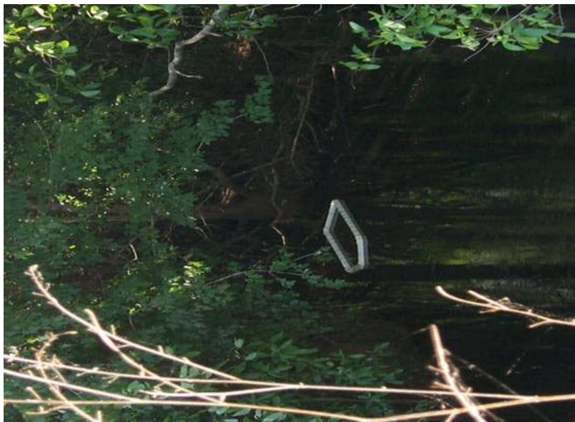
Figure 4.6. Periphytometers deployed in Five Mile Creek (Weber, GA). One frame was deployed in the shade (left) and the other in full sunlight (right).
