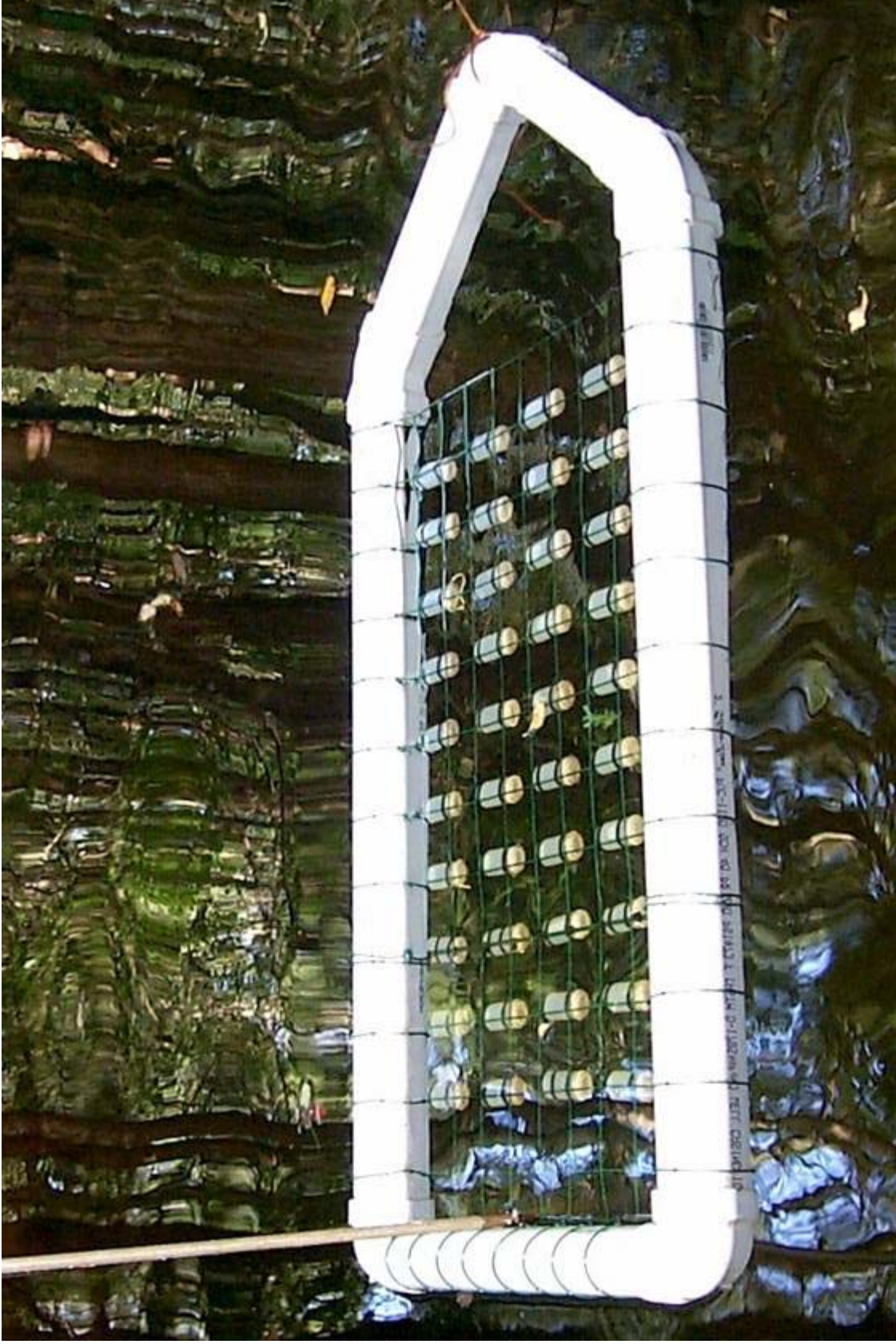
Figure 3.4. Periphytometer frame deployed for September 1, 2003 and October 17, 2003 preliminary experiments. The forty 20 mL scintillation vials are submersed just beneath the water surface.
