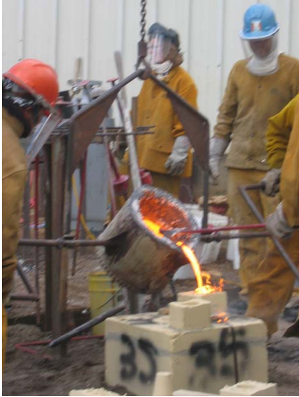
Figure 42: Pouring into the molds
