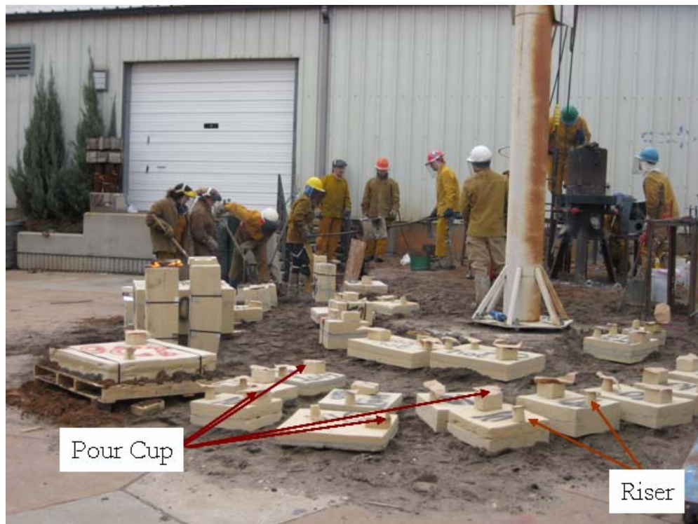
Figure 41: Molds during an iron pour showing pour cups and risers.
