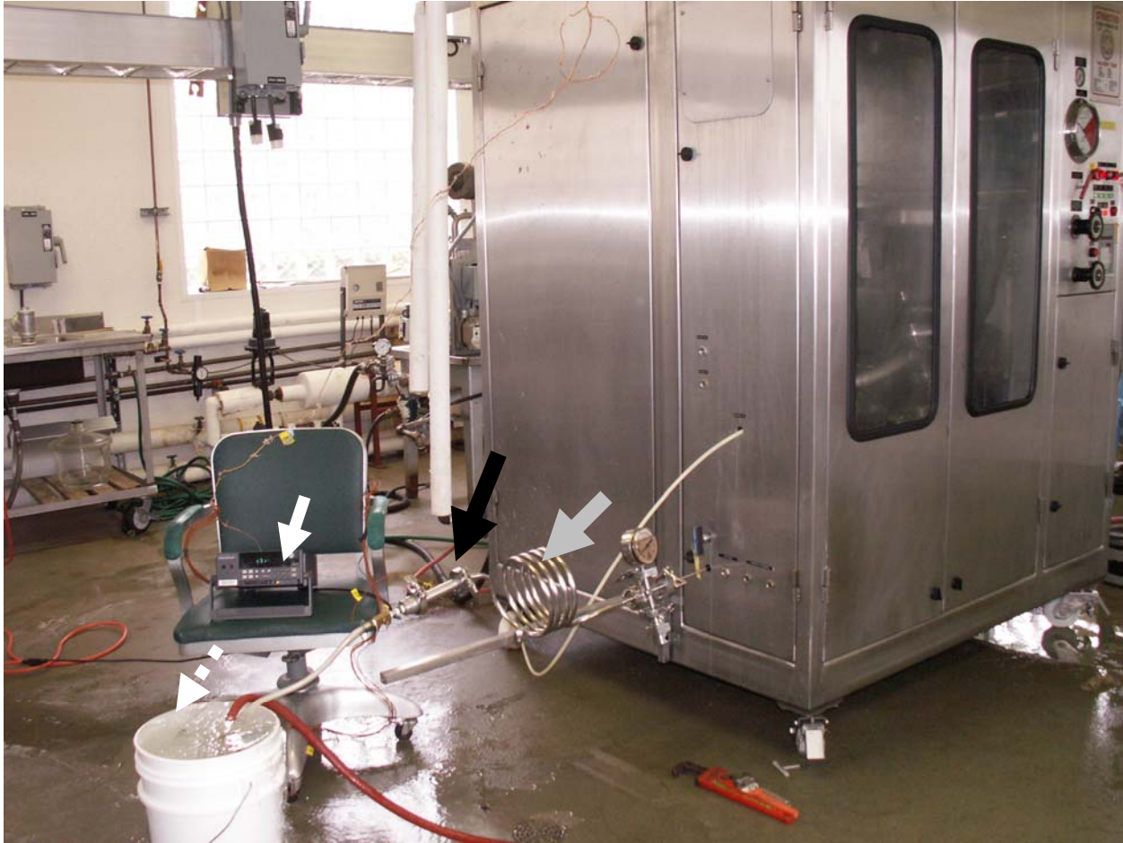
Figure 4.4 – Outside view of Stansted CFHPT system (Model nG7900, Stansted Fluid Power Ltd., Stansted, Essex, UK) with thermocouple attachment to Fluke Hydra Data Bucket (PO Box 9090, Everett, WA 98206-9090). Data bucket (white arrow), holding tube (light grey arrow), thermocouple connected after holding tube (black arrow), and ice bath (white dashed arrow) are shown with arrows.
