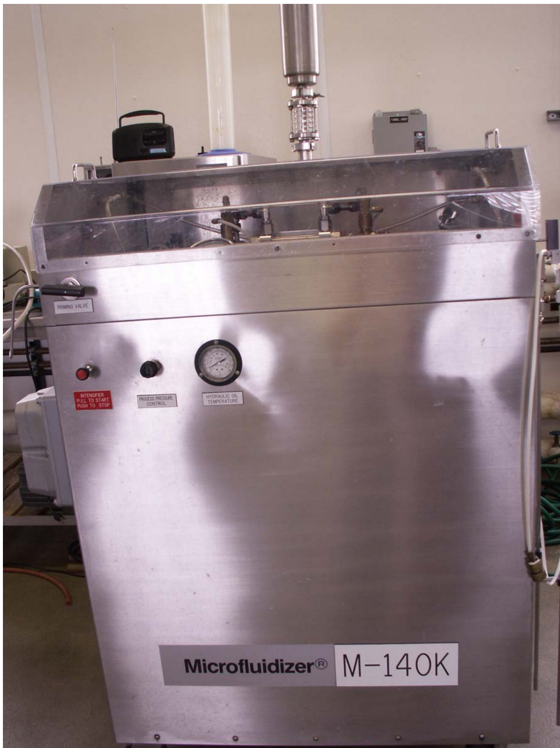
Figure 5.2 – Microfluidizer (outside view) (model M-140K, Microfluidics International Corporation, Newton, Mass.).
