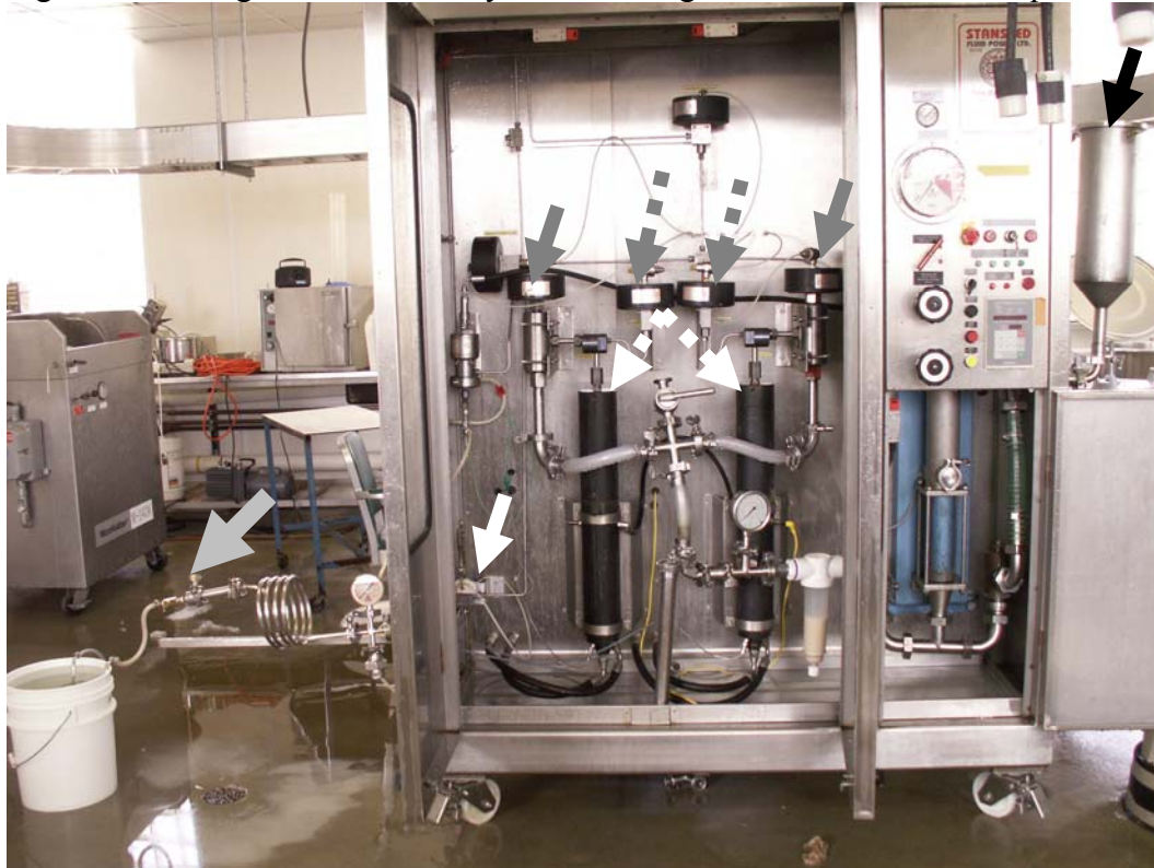
Figure 4.3 – Inside view of Stansted CFHPT system (Model nG7900, Stansted Fluid Power Ltd., Stansted, Essex, UK) with throttling valve (white arrow), intensifiers (dashed white arrows), inlet to CFHPT (black arrow), back pressure valve (light grey arrow), inlet valves to intensifiers (grey arrows), and outlet valves from intensifiers (dashed grey arrows).
