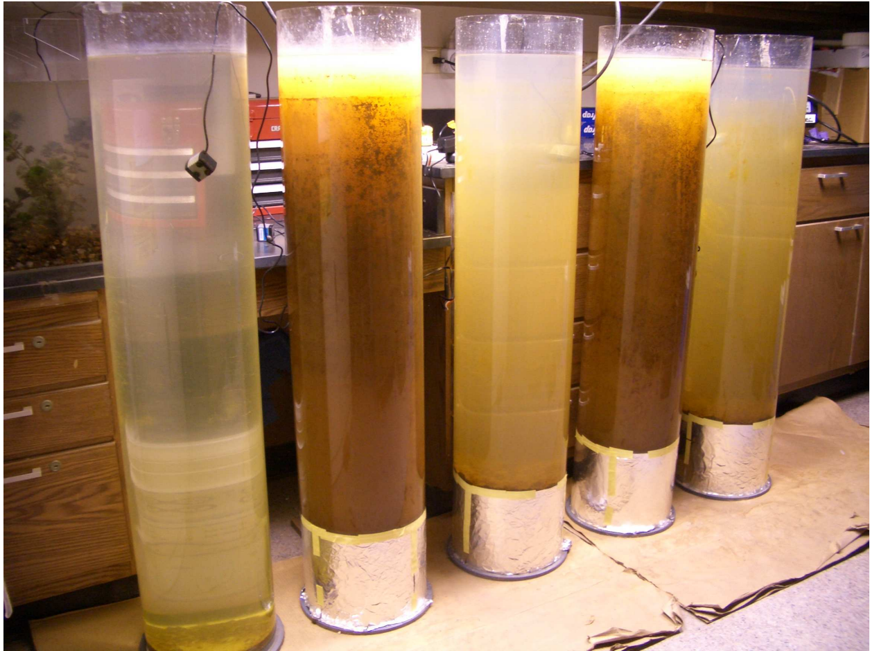
Figure 4.1: Laboratory mesocosm experimental columns (122 cm in height, 26.7 cm in diameter). A control column (left) filled with lake water, while the remaining columns filled with lake water plus approximately 21 cm of lake sediment. Resuspension of sediment in two columns (second and fourth from left) led to increased algal growth.
