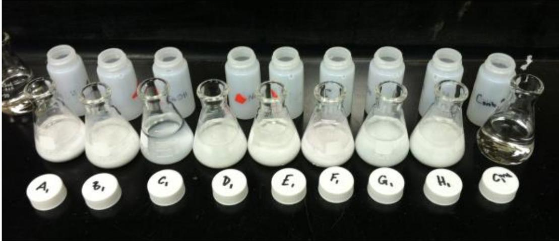
Figure 11. Barium chloride ( $\text{BaCl}_2$ ) was added to the sodium hydroxide ( $\text{NaOH}$ ) to form barium carbonate ( $\text{BaCO}_3$ ) precipitate, the absorbed  $\text{CO}_2$ .
