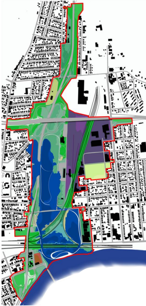
Figure 5.33: Floodable Design 2, 6 Feet above River Bank
