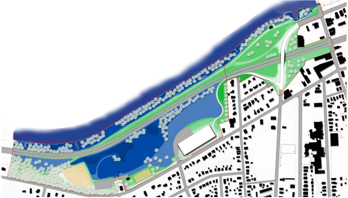
Figure 5.16: Floodable Design 1, 12 feet above River Stage
