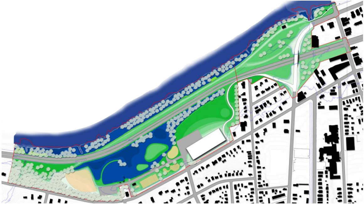
Figure 5.15: Floodable Design 1, 8 feet above River Stage
