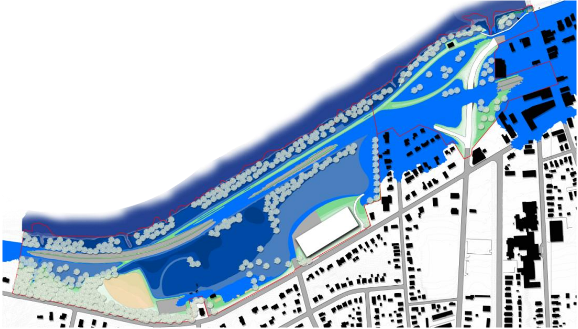
Figure 5.17: Floodable Design 1, 13 feet above River Stage (Approximate 100 Year Flood event)
