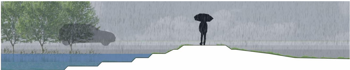
Figure 5.11: Cross-section of Levee during 12 feet above river stage flood
