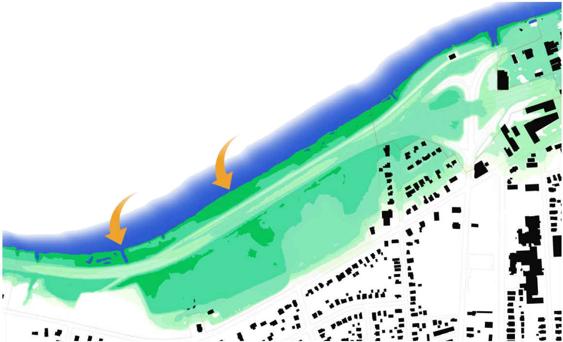
Figure 5.9: Low Points for Potential Levee Openings
