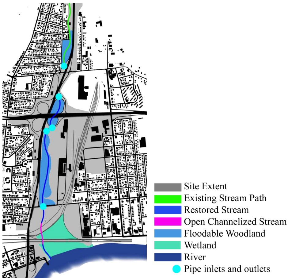
Figure 5.31: Floodable Design 2, Circulation Plan for Stream Daylighting and Wetland
