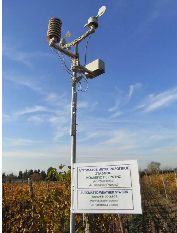
Figure 3.8 Automated Weather Stations were installed in each soil.
