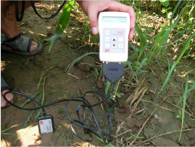
Figure 3.6 The WET sensor and the HH2 datalogger.
