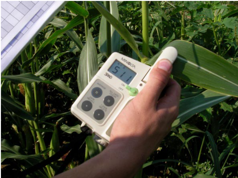
Figure 3.7. The leaf chlorophyll meter (SPAD Minolta 502).
