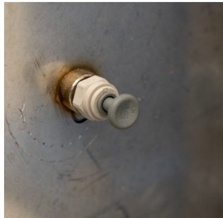
Figure 4.2: One of six pressure taps installed on the HSWT with a removable plug
