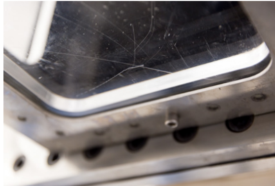
Figure 3.1: Scratches on the bottom acrylic window of the test section.
