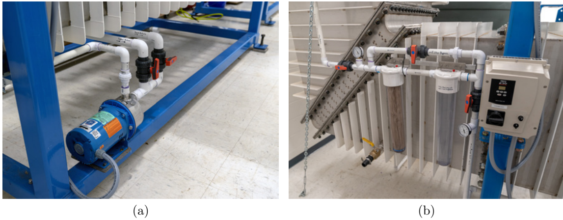
Figure 5.2: (a) Filter pump and manifold (b) Filtration unit
