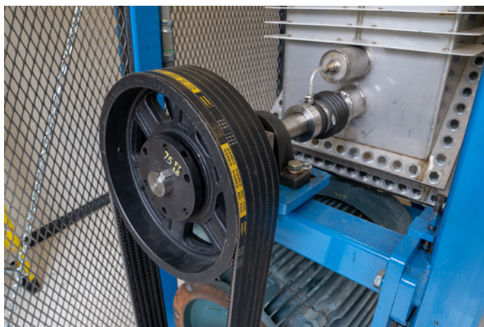
Figure 5.6: Motor belts of the HSWT after one year of use
