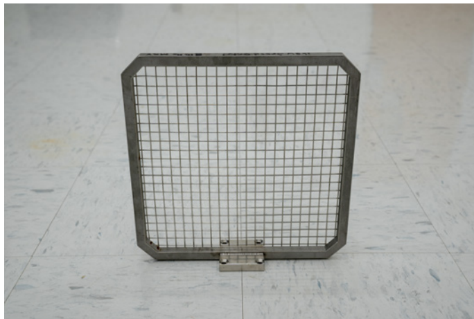
Figure 3.15: The safety bracket designed to fit within the test section and catch stray test articles.
