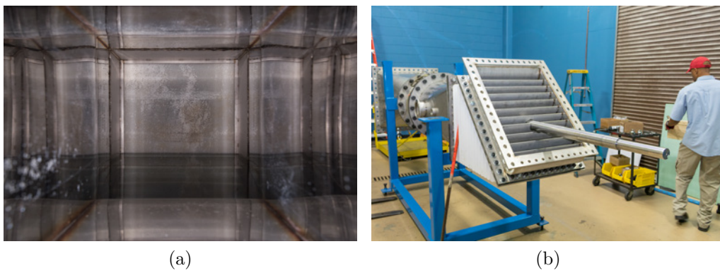
Figure 1.4: (a) Plastic honeycomb matrix and contraction interior as seen from the entrance of the test section (b) One of four sets of turning vanes in the HSWT
