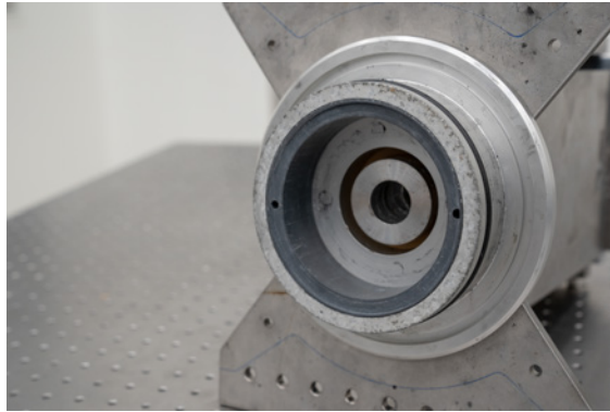
Figure 4.5: PVC retaining ring used to rigidize the force balance
