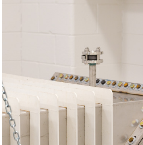
Figure 2.1: The flange and stem assembly added to accept flange-mount pressure-relief discs.
