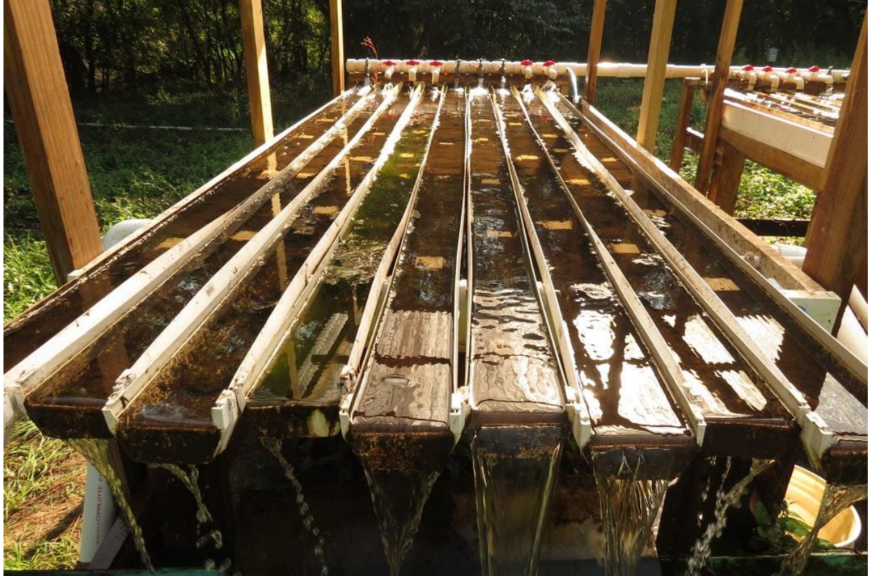
Figure 3.2: Artificial stream channel facility channels made from plastic gutters.
