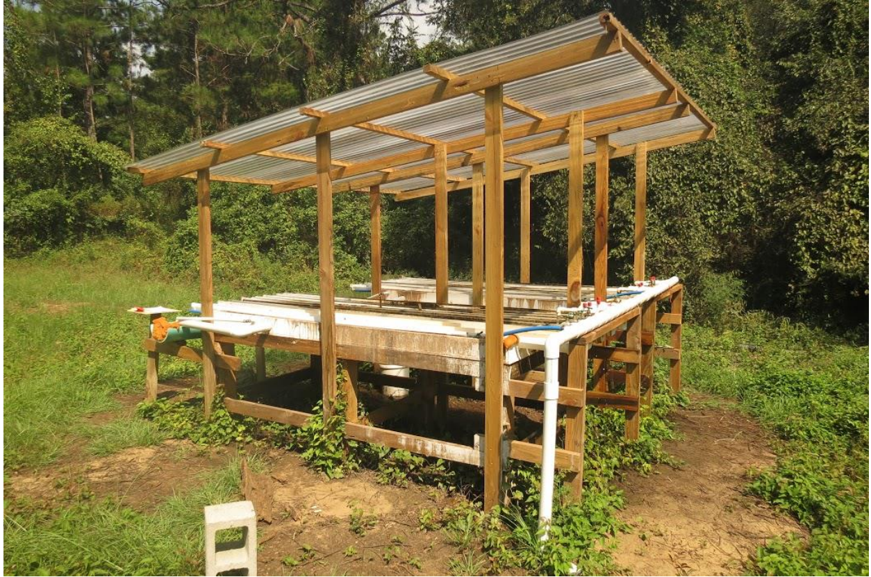
Figure 2.2: Artificial channel system with clear plastic roofing. Water was pumped from the Ichawaynochaway creek and flow treatments were controlled via spigots.
