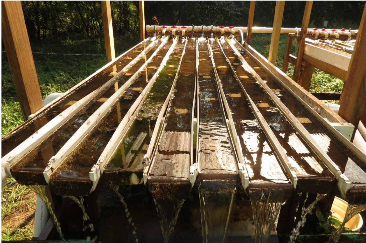
Figure 2.3: Artificial stream channels (width = 6 inches, length = 10 ft) on top of a flow-through water bath.
