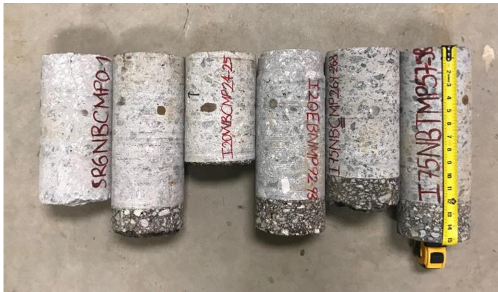
Figure 6.1– Core Specimens taken from Site Investigations
