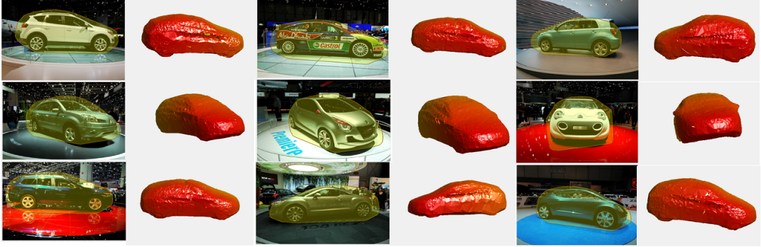
Figure 3.4: Qualitative results. Left : Test images overlaid with the projection (2D convex hull) of the estimated shape and viewpoint. Right : Full 3D reconstruction of the test object instance obtained by deforming basis shapes (meshes) using estimated shape parameters rotated to the estimated pose.
