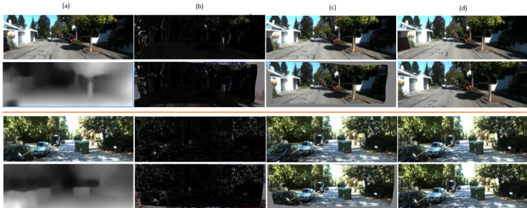
Figure 5.5: (a) Target image and its estimated depth map, (b) left and right photoconsistency error, (c) Projected left and right images (d) groundtruth left and right images.
