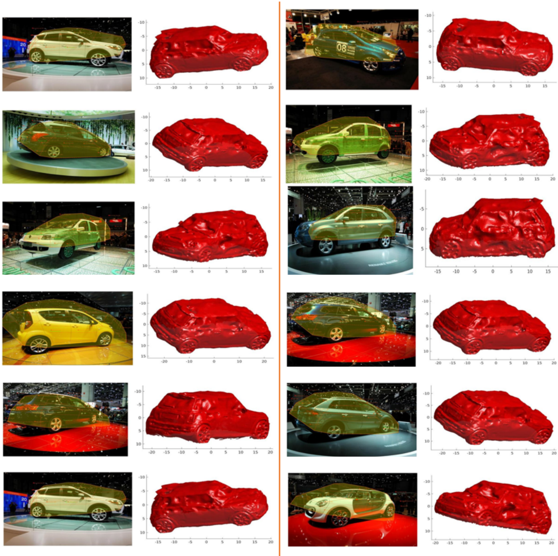
Figure 2.5: Qualitative results of the proposed RANSAC -based Viewpoint Estimation and Shape Recovery, on EPFL Multi-view Car dataset. Odd columns illustrate the test image with corresponding Viewpoint/Shape estimations overlaid on it. Even columns illustrate the Viewpoint Estimation of their corresponding test image (on its left), using a sample mesh (from our dataset) for better visualization. ( note : meshes (in even columns) are not generated/reconstructed by our viewpoint estimation approach, and are used only for the purpose of better visualization in all our qualitative results).
