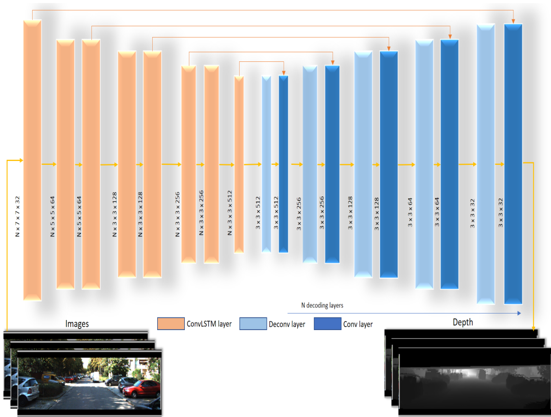
Figure 4.1: Proposed network architecture: The encoding layer consisting of multiple ConvLSTM [31] layers (orange blocks) takes a single image or image sequence as input at test time. The decoding layer consisting of an alternating sequence of deconvolutional and convolutional layers ( blue blocks ) reconstructs the depth maps.
