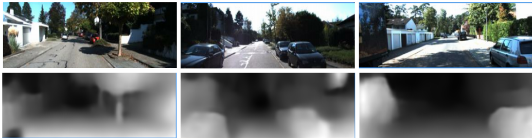
Figure 5.4: Qualitative results of depth prediction on KITTI dataset, where the network is trained in an unsupervised manner. Top row consists of target images and the bottom row consists of the corresponding predicted depth maps.
