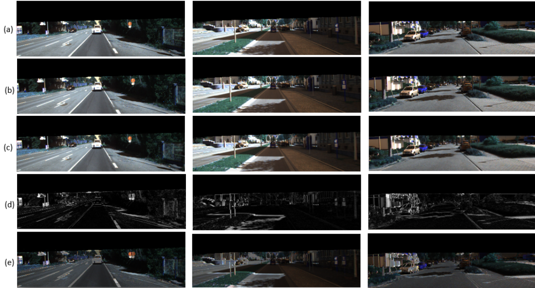
Figure 5.3: (a) Source images ( left ( I_{t-1} ) or right ( I_{t+1} )) (b) Target image (c) Generated (transformed source) image, using the estimated pose and depth parameters (d) photoconsistency error between generated ( c ) and ( b ), (e) Adversarial example with induced photoconsistency loss. The discriminator is trained with images in ( a ) and ( b ) as real vs. images ( e ) as fake. Image ( e ) has been enhanced with higher values of \omega ( =0.6 ) to amplify the difference for visual demonstration, but during training, the induced photoconsistency loss is kept lower.
