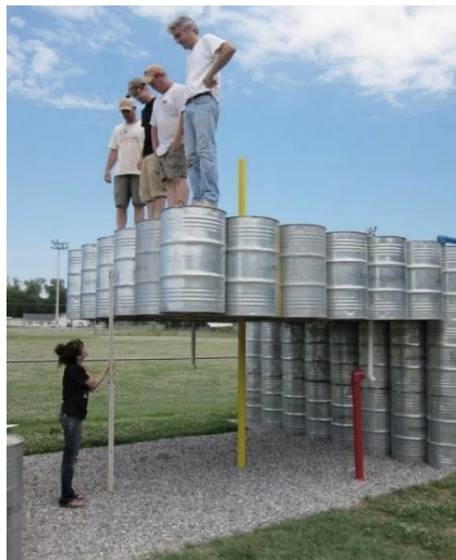
Figure 50: The load test for the barrel roof: The roof can hold 3200 pounds (LionsParkscape 2010).
