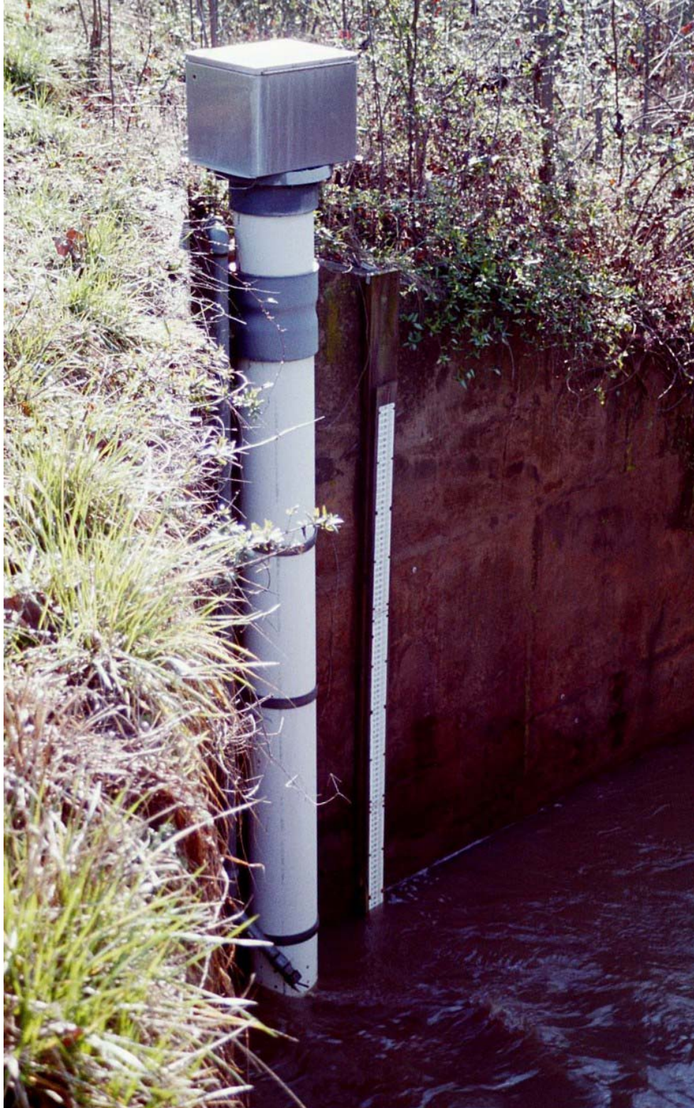
Figure 4.6. Staff gage used for determining flow in West Fork Little River at Jess Helton Road, attached to the southeast culvert wing wall by USGS.
