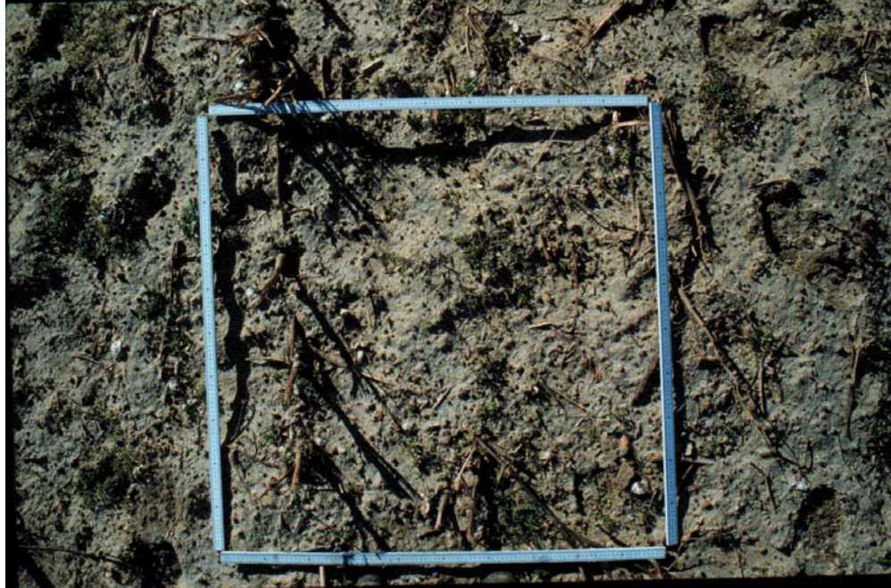
Figure 4.12. Vertical photograph at Subwatershed K ground truth point 4 with meter sticks placed in an approximate square for scale.
