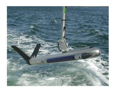
Figure 4.8. Klein 3000 Dual Frequency Single Beam Side-scan Sonar. Source: Klein Associates, Inc.
