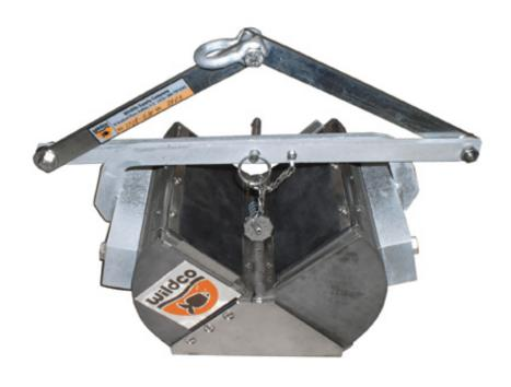
Figure 4.9. Wildco Ponar Grab Sampler. Source: Wildlife Supply Company.
