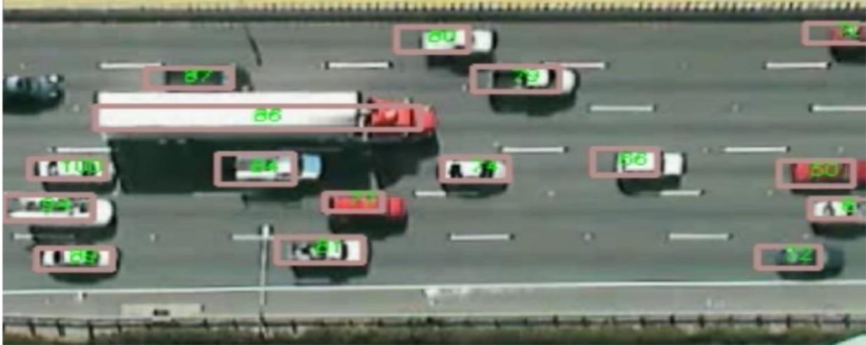
Figure 5.3: Snapshot of the processed video from NGSIM I-80 freeway merging study. The processing of video helped in detecting all the vehicles in each frame and assigned them unique IDs.
