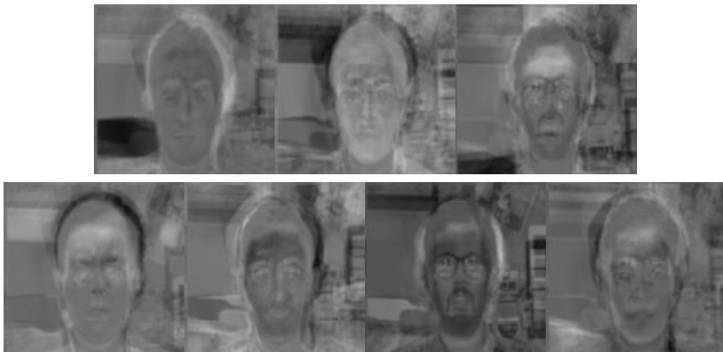
Figure 2.7. Seven of the eigenfaces calculated from the images of Figure 2.5, without the background removed [6]. (With kind permission of MIT Press Journals)
