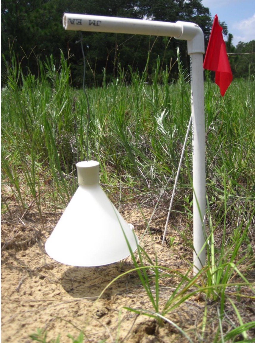
Figure 3.5. The environmental station setup for collecting shaded ambient air temperatures on the surface using a design adapted from Hubbart (2011). The ambient air temperature logger was secured 10 cm above the ground's surface. It was placed approximately 30 cm away from the entrance to the abandoned burrow.
