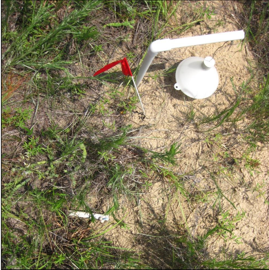
Figure 3.4. The environmental station was setup to collect both ambient air temperatures on the surface as well as air temperatures in an abandoned juvenile gopher tortoise burrow. The ambient air temperature logger was secured 10 cm above the surface using a design adapted from Hubbart (2011). It was placed approximately 30 cm away from the entrance to the abandoned burrow where burrow temperatures were taken. The temperatures of the inside of the burrow were taken with a temperature logger secured to the end of a PVC pipe and placed approximately 1m inside the burrow. A small portion of the end of the PVC pipe remained visible at the entrance to the burrow.
