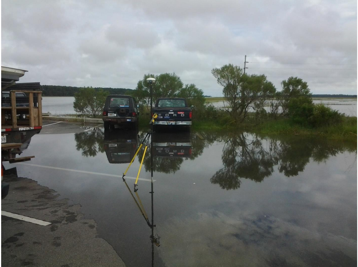
Figure 4.2 RTK GPS. Elicitation technique and accuracy assessment of elevation data. Photo is of the nuisance flooding in the parking lot caused by high tide at 10:23 AM at Sapelo's Marsh Landing on September 29, 2015. The nearest NOAA tidal gauge is at Fort Pulaski (~ 80 km to the northeast); it recorded high tide of 2.993 m at 9:54 AM relative to the station's mean lower low water datum. This day's recorded high tide was 0.706 m above the station's mean higher high water datum.
