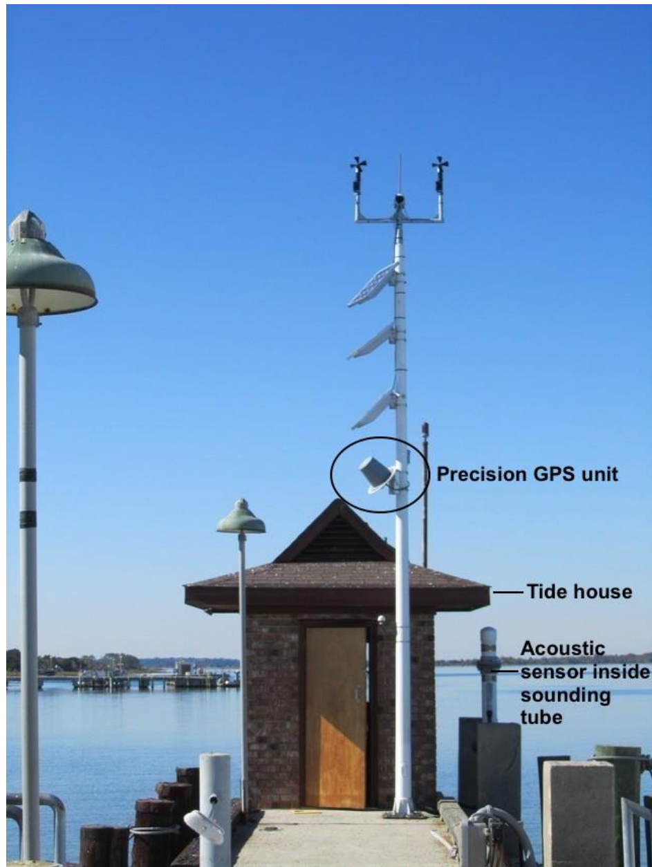
Figure C.4 Recent photograph of Fort Pulaski tide gauge located on the Savannah River. Photo credit: NOAA's CO-OPS ( http://tidesandcurrents.noaa.gov/ , accessed 7/19/2016). To learn more about how CO-OPS measures water levels, visit http://oceanservice.noaa.gov/education/tutorial_tides .
