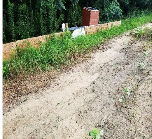
(b) CT Flume after a rainfall event, where there is evidence of runoff in the freshly deposited sand
