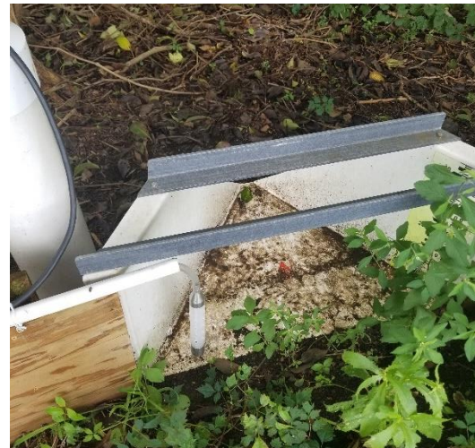
(b) ST H-flume after a rainfall event, with no runoff indication
