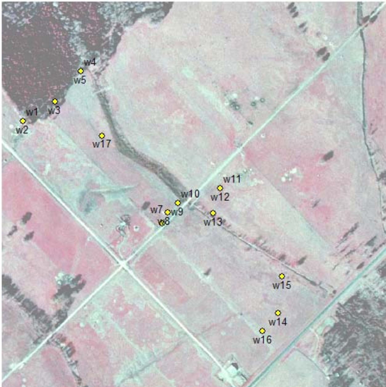
Fig. 4.7. Piezometer locations on project site. Wells 1, 2, 14, 15, and 17 were equipped with data loggers that took daily readings. Remaining wells were manually read weekly.
