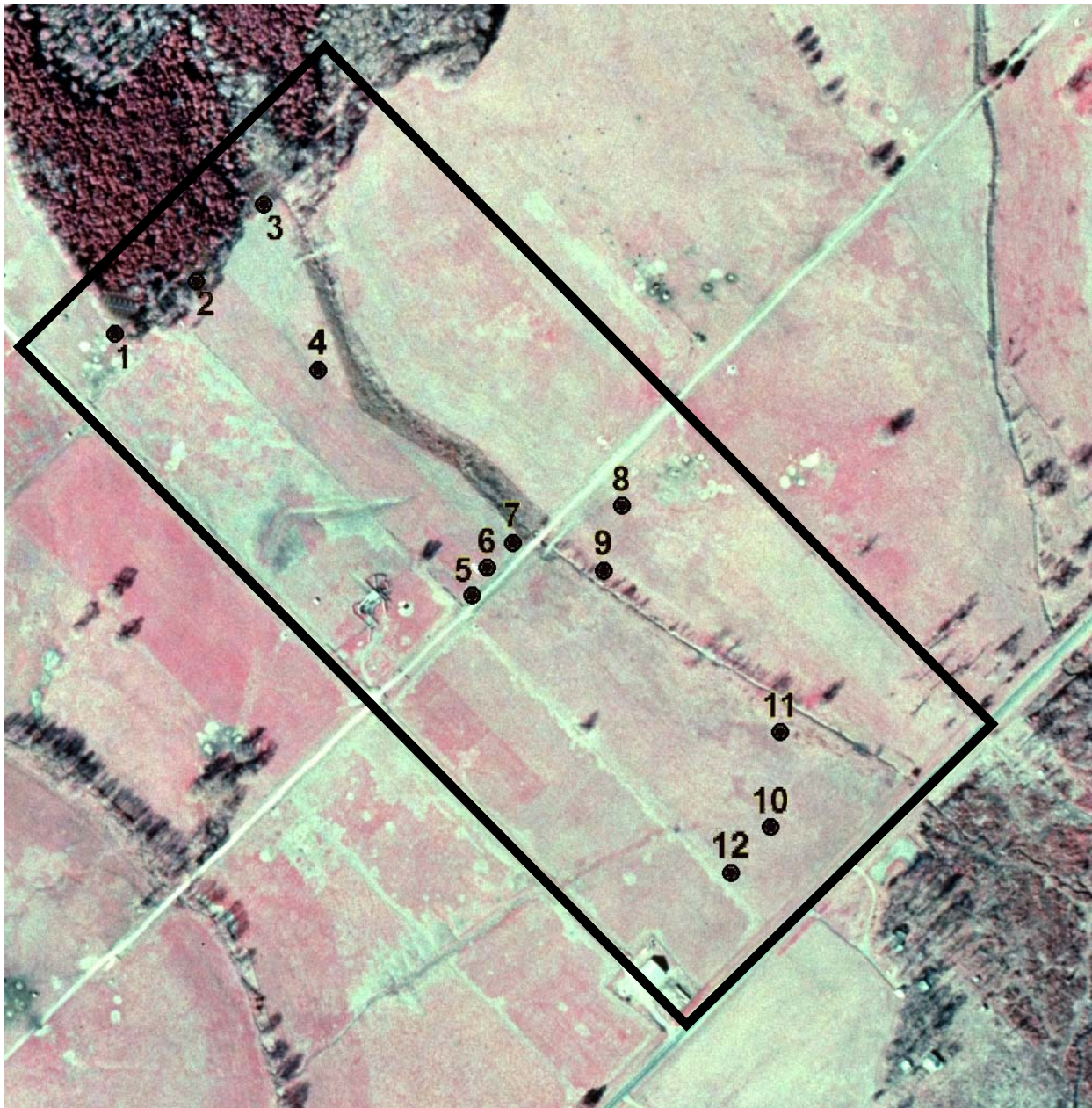
Fig. 3.2. Piezometer locations on project site. Sites 1, 4, and 11 were equipped with well dataloggers, Pt electrodes, and IRIS tubes. Additionally, sites 3, 6, 7, 9, 10, and 12 were equipped with IRIS tubes.
