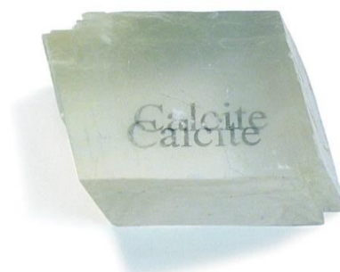
Figure 1.4: Optical birefringence shown in a calcite crystal
