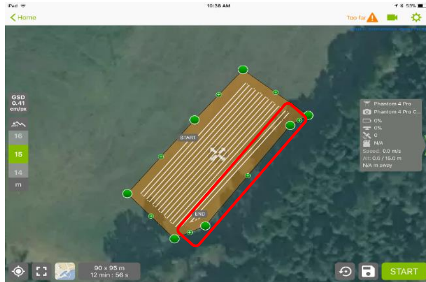
Figure 19: Flight plan in PIX4D interface using an iPad as flight controller for Phantom 4 Pro. The portion highlighted in red was flown manually due to proximity of trees.
