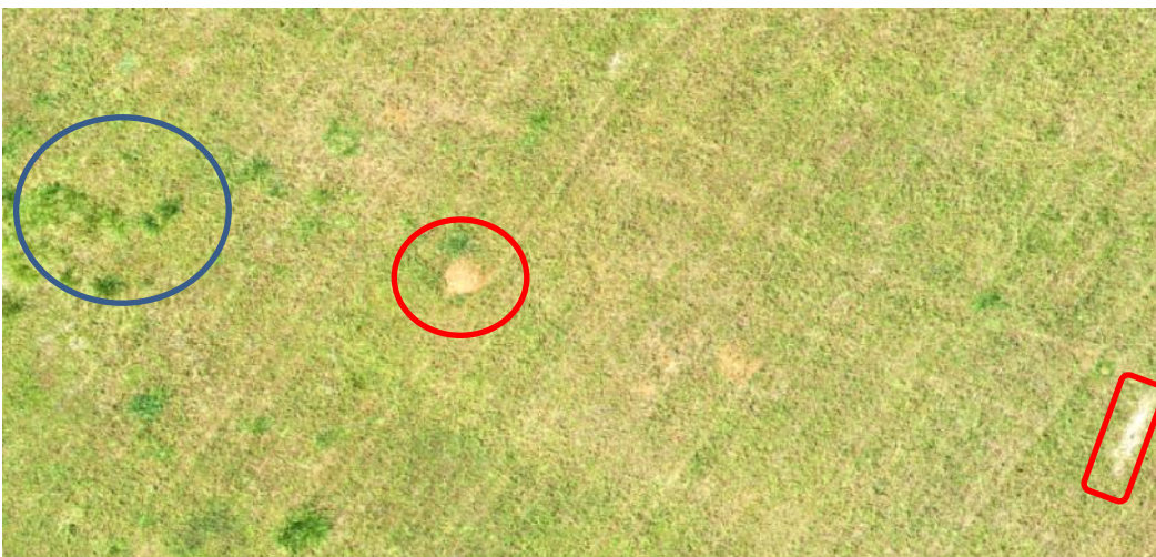
Figure 15: Close-up of study site B taken from April 20 th orthomosaic - Grass clumps are common and occur as circular features. Red -Dirt features can occur as circular or linear.
