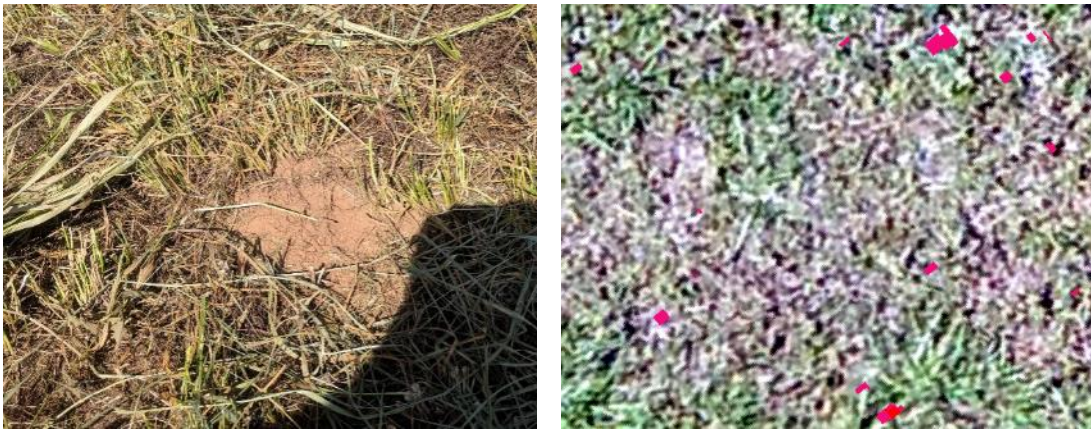
Figure 26: Left - Examples of grass shoots and dirt patches that were incorrectly identified as anomalies and possible simulation landmines. Right - April 20 th P4P orthomosaic overlaid anomaly detections showing grass and dirt have been incorrectly identified.
