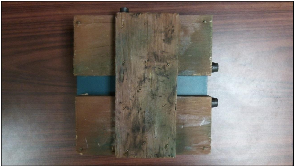
Figure 2-5. Platform fitted to the back of the Song Meter SM2 to facilitate attachment of the unit to trees on the Joseph W. Jones Ecological Research Center and Silver Lake WMA in southwestern Georgia, USA, 2011-2012.
