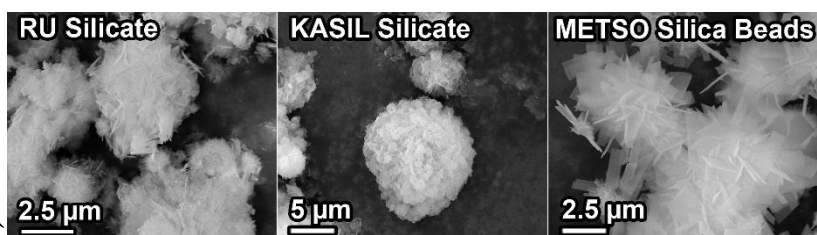
Figure 4.11. Morphology change of \text{BaCuSi}_4\text{O}_{10} when varying silica starting material run at 250 °C for 48 h.
