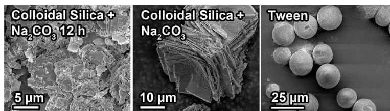
Figure 4.8. Morphology change of the \text{SrCuSi}_4\text{O}_{10} crystals when the baseline synthesis was run at 250 °C for 48 h with various additives.
