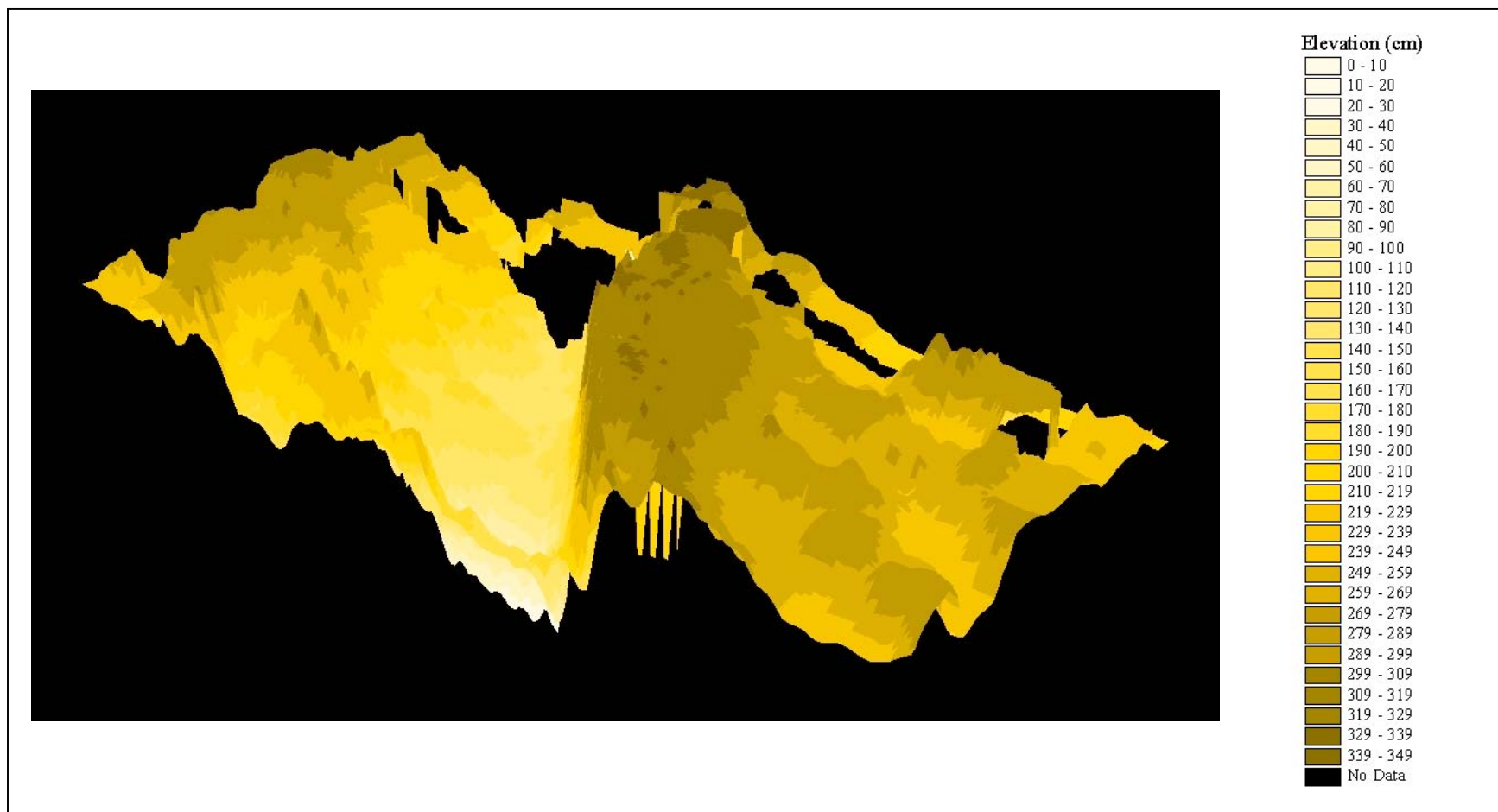
Figure 2.14: Example digital elevation model (DEM), depicting topography on plot A. The x and y axes, which depict the perimeter of the plot, are measured in meters. The z-axis, which represents elevation, is measured in centimeters. Black denotes areas with no elevation data.
