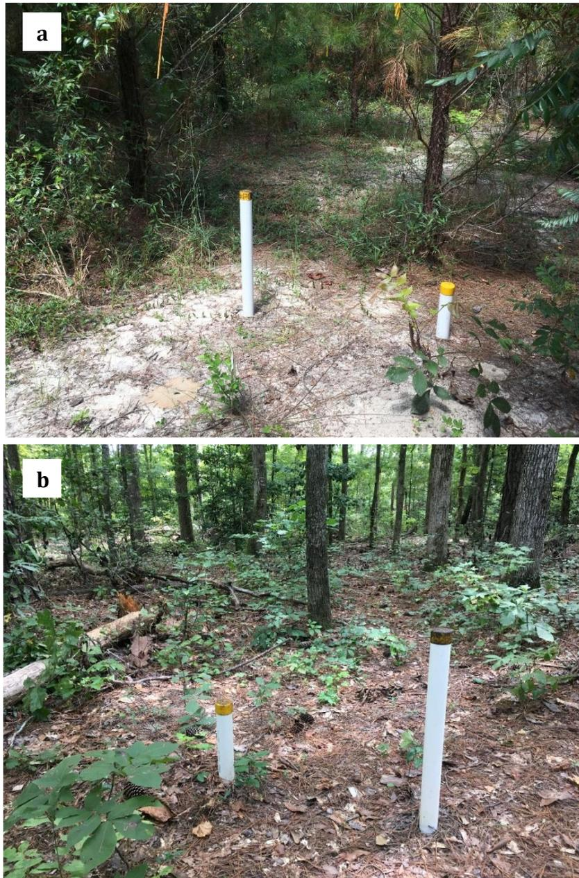
Figure 3.6: Examples of nested wells installed to monitor the establishment of a perched water table above an argillic layer commonly found in the Fourmile Watershed: (a) W03 & W03D located on the hillslope of the short rotation pine plantation, and (b) W11 & W11D located on the forested hillslope within the SMZ.
