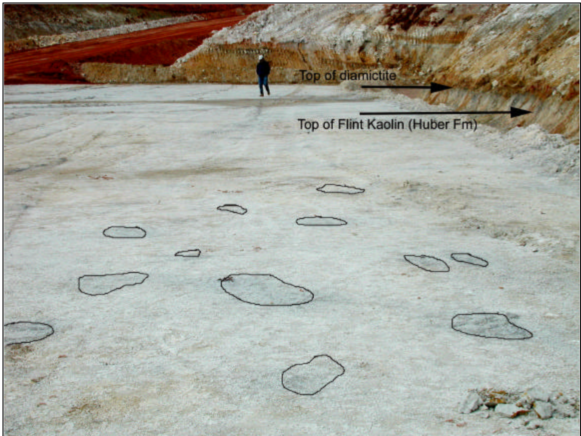
Figure 48. Photograph (contrast-enhanced) of large stump holes in the top of the Huber Formation uniformly filled with the diamictite breccia. Only a small number of the observed holes are outlined in the image. Note thesis advisor for scale (approximately 1.7 meters tall).
