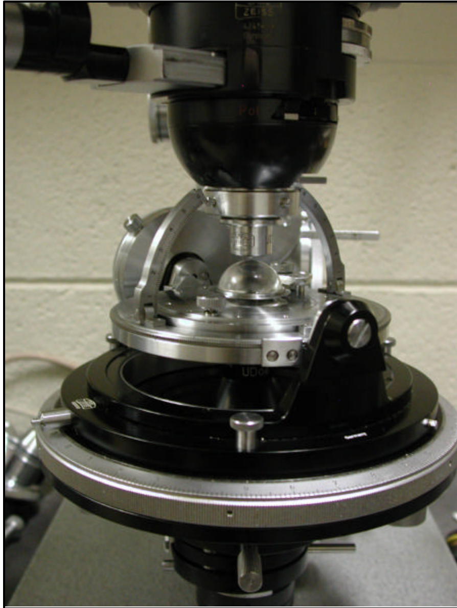
Figure 14. Photograph of a Zeiss four-axis universal stage used to measure the orientation of quartz micro-fabrics. A thin section or grain mount is placed flat between two glass hemispheres (the upper hemisphere is visible near the center of the photograph).
