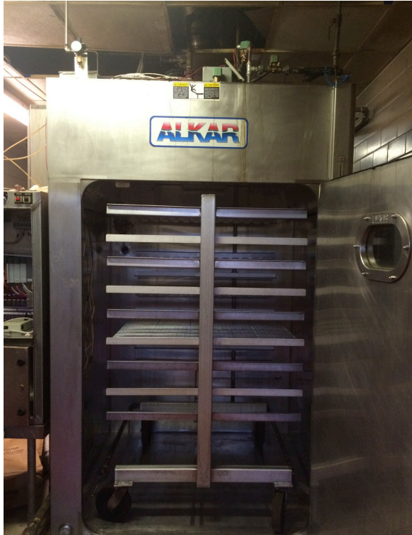
Figure 2.2 ALKAR TM (Lodi, Wisconsin) Forced-ventilation Smokehouse
