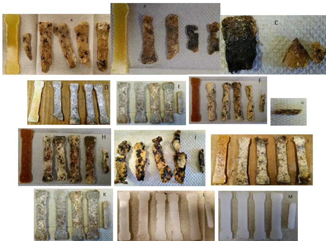
Figure 4.8. Plastics that have been subjected to biodegradation susceptibility analysis: (a) Albumin-Glycerol (30 Days); (b) and (c) Albumin-Glycerol-5 LDPE (30 and 60 Days); (d) and (e) Albumin-Glycerol-50 LDPE (30 and 60 days); (f) and (g) Zein-Glycerol (30 and 60 days); (h) and (i) Zein-Glycerol-5 LDPE (30 and 60 Days); (j) and (k) Zein-Glycerol-50 LDPE (30 and 60 days); (l) and (m) LDPE (30 and 60 days)
