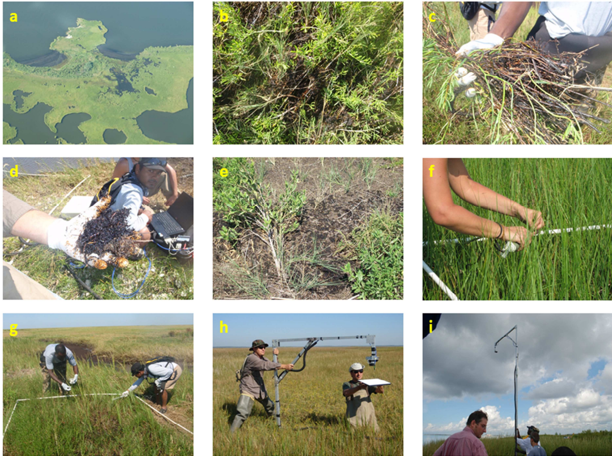
Figure 2.2. 2010 Field Research Photographs: (a) Resident oil observed through airplane survey; (b, c, d, and e) Oil observed in vegetation canopy and root system, and soil; (f) Leaf chlorophyll reading using SPAD; (g) LAI reading using LICOR's LAI-2000 meter; (h) In situ sensor calibration; (i) In situ remote sensing data acquisition
