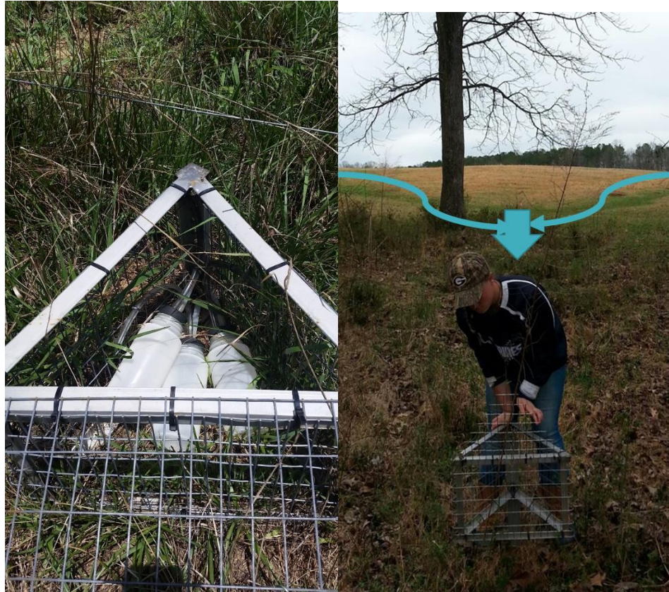
Figure 3.6. The photo on the left shows the set up for the Poore-point runoff collectors placed at the edge-of-field in order to collect runoff. The tubing creates a vacuum system that slowly collects water at different runoff heights during and after a runoff-producing rainfall event. The photo on the right demonstrates the placement of the runoff collector within the pasture. The blue arrows demonstrate a concentrated flow pathway.
