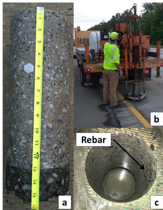
Figure 7.6 - Typical Cores at Rebar Locations (a) Core sample; (b) Coring machine; (c) Inside view of a cored pavement.
