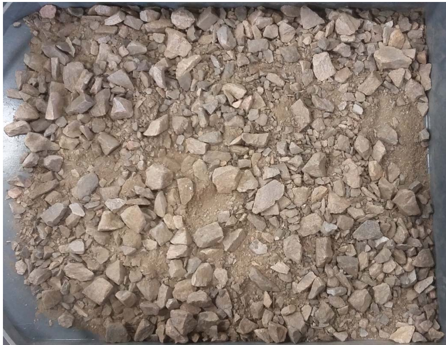
Figure 8.9 - Asphalt Sample after Ignition Burning
