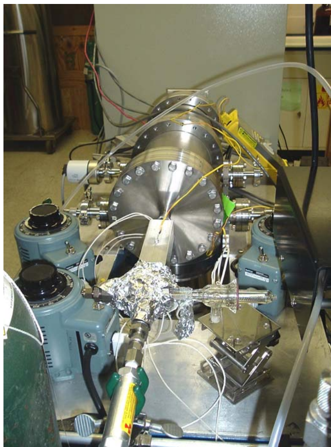
Figure 2.2. Photographs of the vaporizer (top) and the entire aerosol chemical ionization mass spectrometer system (bottom).
