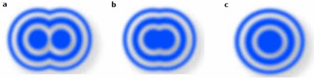
Figure 1.4: These images demonstrate the Rayleigh criterion. (a) Two point sources of light that are neighboring one another, yet have a far enough distance apart that they may be individually resolved. (b) The same sources but are now only just resolved by a minimum required distance to distinguish between two points. (c) Two points completely overlaid upon one another reaching the resolution limit [4].
