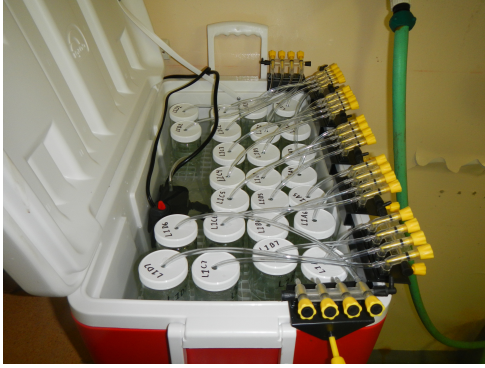
Figure S4.1. Experimental setup, with 20 jars each containing an E. depressus , fit with an airstone connected to an aerator. To maintain a constant temperature for the whole cooler we placed a single pump head next to an aquarium heater that was isolated some distance from the experimental jars.
